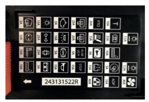
1. Identify ignition (+) fuse circuit i.e. radio. DO NOT connect to any primary vehicle safety systems.
