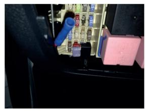
4. Insert fuse jumper into fuse box.
