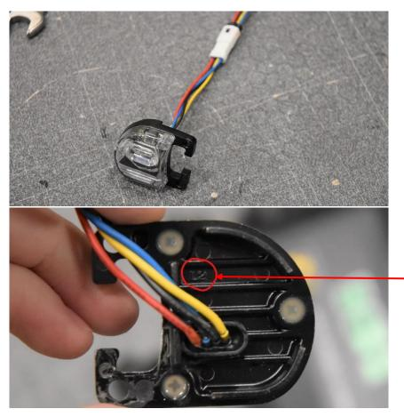
The lights are marked with L or R Pull the loose end cable through the hole and rest of the cabling in the roof bar.
