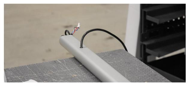
Connect the lights with the cable and screw them on the roof bar.
